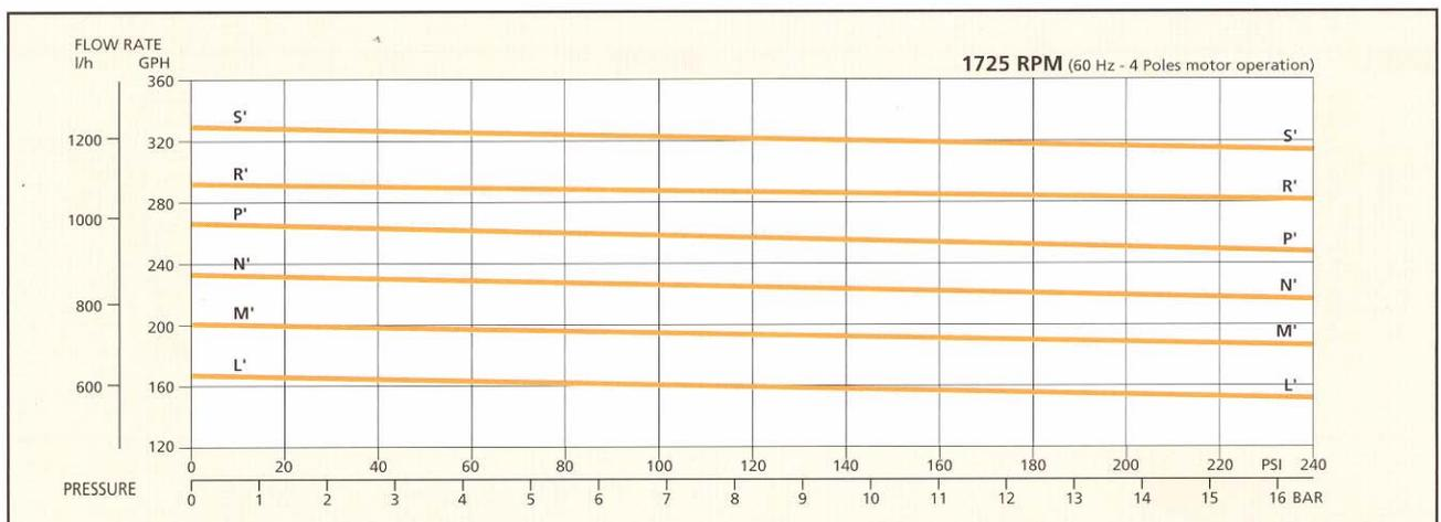
Characteristics at constant motor speed, with water at 68 °F and by-pass blocked - Figures of flow are averages - Pump weight: 1,9 kg (4,2 Lbs) clamp mount and 2 kg (4,4 Lbs) flange mount
