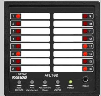
AFL100 is an alarm annunciator, intended to replace the lamps on the frontage of cabinets and which integrates all the functions necessary for local or remote signaling: memorization, blinking, acknowledge and alarm. Directly embedded, it can be mounted on a rack, on a reading desk or in a cabinet. Different options allow a fully adaptation: number of inputs, of relay outputs and a communication link available with different protocols.
